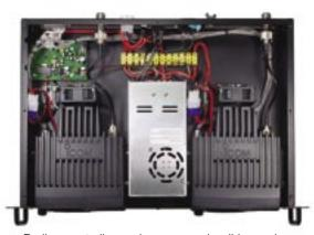
Radios, controller, and power supply, all in one box. Dual forced-air fans keep the unit cool. 19" Rack mountable. Battery backup capable.
